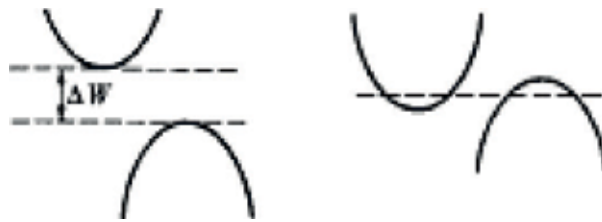
Figure 3. Two Hubbard bands overlapped in metal case, and not overlapped in insulator non-metal.
