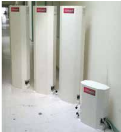
Figure 13. Photography of the RPM prototype (Katrina) developed by the CEA in the framework of the SECUR-ED project funded by the European Commission [30].
