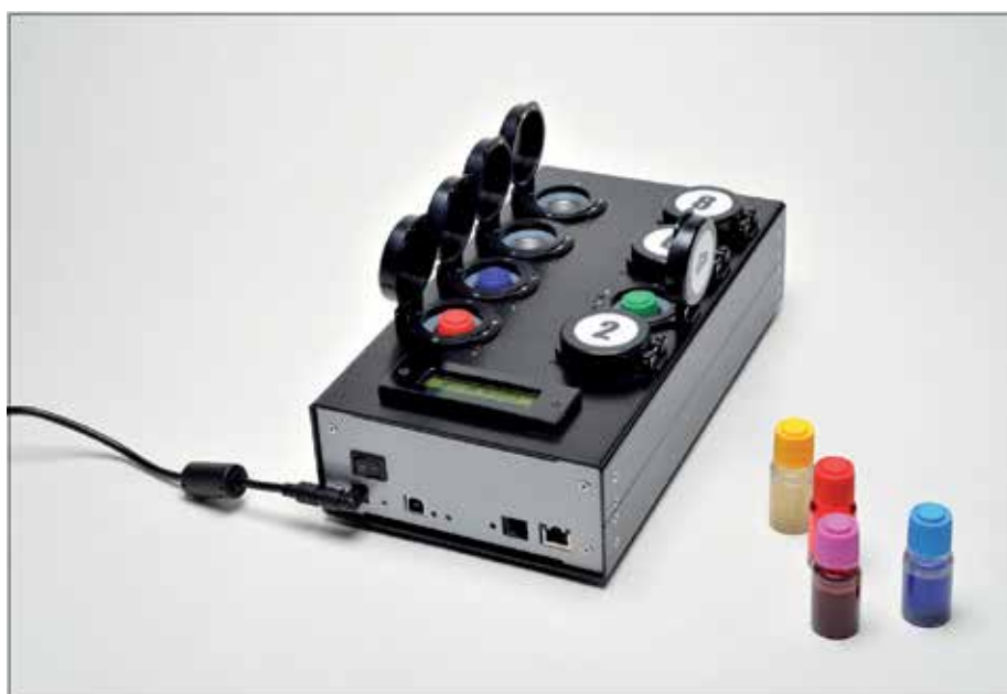
Figure 1. MBS "UTI CHECK." MBS "UTI CHECK" is an automated colorimetric culture-based test. It is composed by mono-use, disposable and ready-to-use reaction vials (right) in which 1 ml of urine can be inoculated without any preliminary treatment. Up to eight urine-inoculated reaction vials can be independently allocated in an automatic thermostated optical reader (left) that it is able to detect color change induced by the growth of bacteria and automatically correlates the time required for color change with the number of bacteria present in the urine samples. Different vials contain selected antibiotics and the occurrence of the color change in the presence of antibiotics indicates antibiotic resistance of bacteria present into the urine sample.
