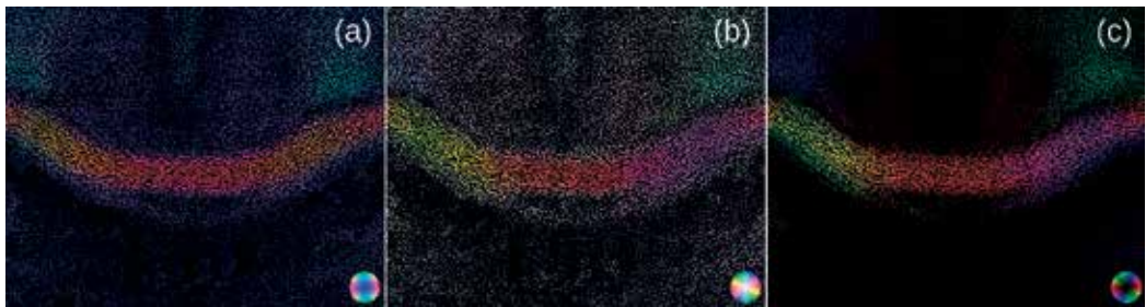
Figure 5. The color-coded glyphs are shown in the RGB color space (a), in the HSV color space (b), and in a special HSV color space: HSV black (c). The colored spheres in the lower right corner of every image are used as legends.
