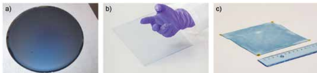
Figure 3. Examples of substrates treated via PRAP-CVD to obtain PEDOT films: (a) silicon wafer (20 cm in dia), (b) glass (15 × 15 cm 2 ), and (c) PET fabric (12 × 12 cm 2 ) [41, 44].
