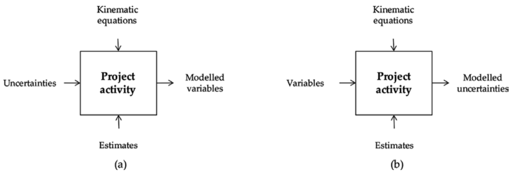
Figure 5. (a) Direct kinematic model and (b) inverse kinematic model.
