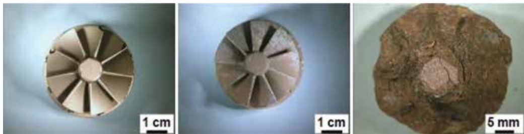
Figure 20. Macroscopic images of the second untreated TiAl rotor with a different chemical composition before (a), after 100 h (b), and totally destroyed after 1200 h (c) of oxidation at 1050°C in laboratory air.
