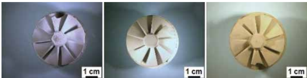
Figure 21. Macroscopic images of an F-treated turbocharger rotor after spraying (a), after 100 h (b), and 1200 h (c) of oxidation at 1050°C in laboratory air.
