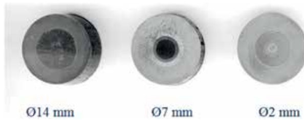
Figure 20. Cross sections of the bars formed in the hot hydrostatic extrusion process.
