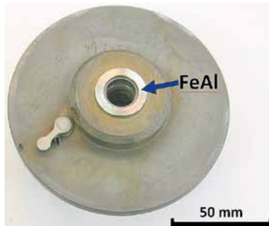
Figure 17. Turbine lid. The arrow indicates the sealing made of the alloy based on FeAl intermetallic phase matrix.
