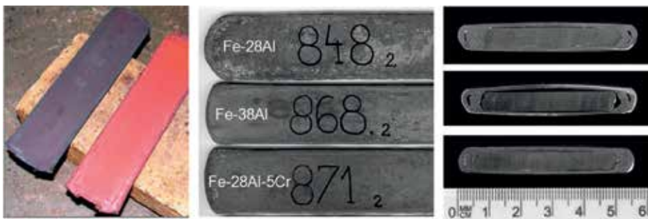
Figure 15. Views of the profiles after rolling with total reduction of ~70% to a thickness of 6 mm.
