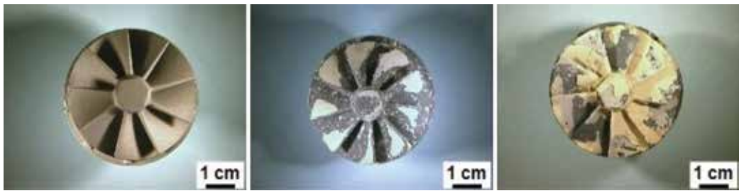
Figure 19. Macroscopic images of an untreated turbocharger rotor before (a), after 100 h (b), and 1200 h (c) of oxidation at 1050°C in laboratory air.
