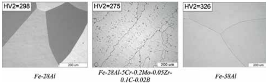
Figure 8. Microstructures of the studied alloys after the high-temperature annealing for 24 h and oil cooling.
