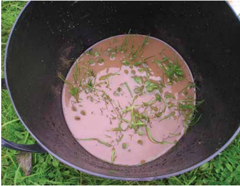
Figure 4. A bottomless container was embedded into the soil surface of a floodplain and 200 g of ^{60}\text{Co} -labelled sediment, mixed in 25 l of water, were poured into the container and allowed to infiltrate, thereby depositing the labelled sediment onto the soil surface under simulated flood conditions.
