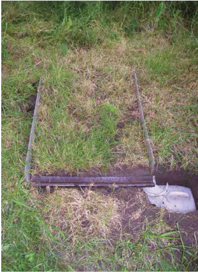
Figure 7. A number of ^{60}\text{Co} -labelled earthworm casts were spread across a bounded area of pasture and exposed to natural weather events for 76 days.
