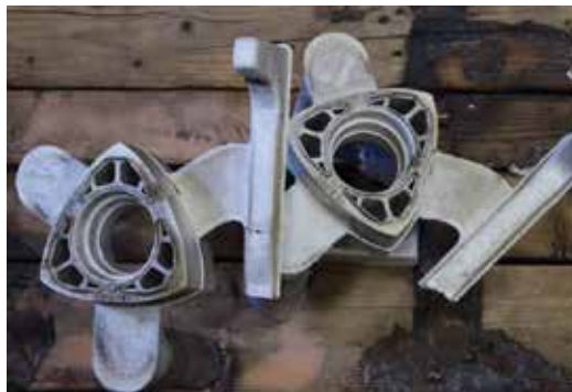
Figure 8. Experimental rotary engine rotor produced in chemically bonded sand with an Al-Ce-Mg alloy.
