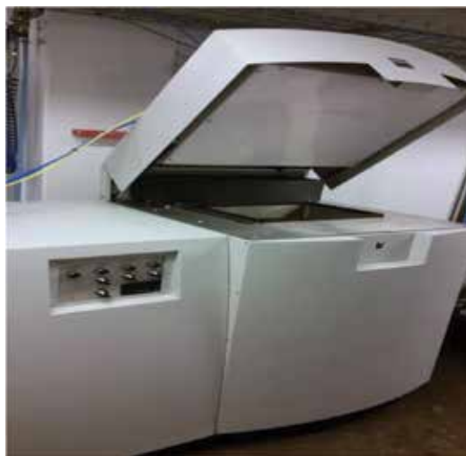
Figure 2. Netzsch™ IBC 284 isothermal calorimeter used in the chapter for measuring the thermal behavior of battery cells.
