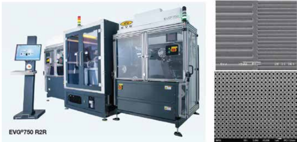
Figure 13. Photo of the EVG750 ® R2R hot embossing system, imprinted, SEM image of 10 \mu\text{m} and 30 \mu\text{m} microfluidic structures replicated into PMMA, 500 nm holes replicated into PMMA [31].
