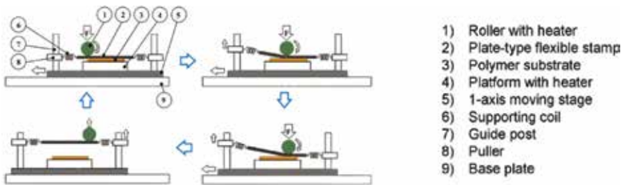
Figure 5. Process flow chart of the roller-based NIL process [22].
