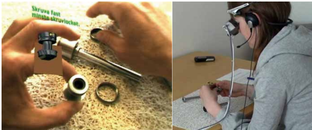
Fig. 8a) The participant's view in the HMD. b) A participant wearing the head mounted display and using the headphones and voice interaction to follow the AR instructions.
