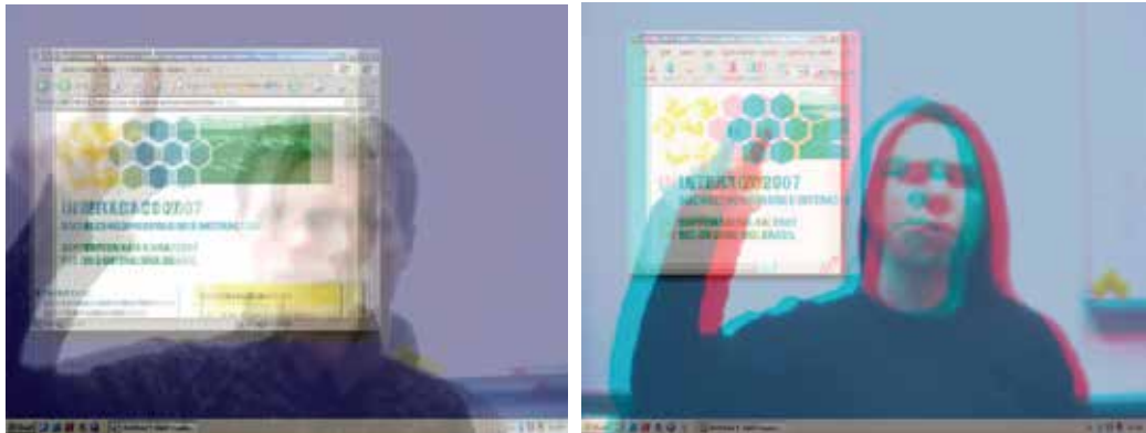
Fig. 2. Screenshot of an AS desktop overlaid with a transparent image of the user in (left) vertical interlaced mode and (right) anaglyph mode.
