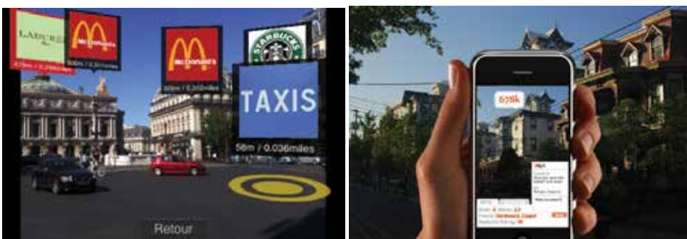
Fig. 2. Examples of augmented reality wherein live video is annotated with information such as nearby eateries, taxi stand, house on sale etc.
