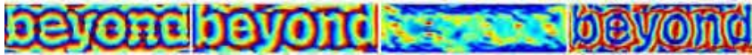
Fig. 8. Log-Gabor filtering results for each filter property. From left to right: phase of the horizontal filter, phase of the vertical filter, magnitude of the vertical filter and absolute phase of the vertical filter.
