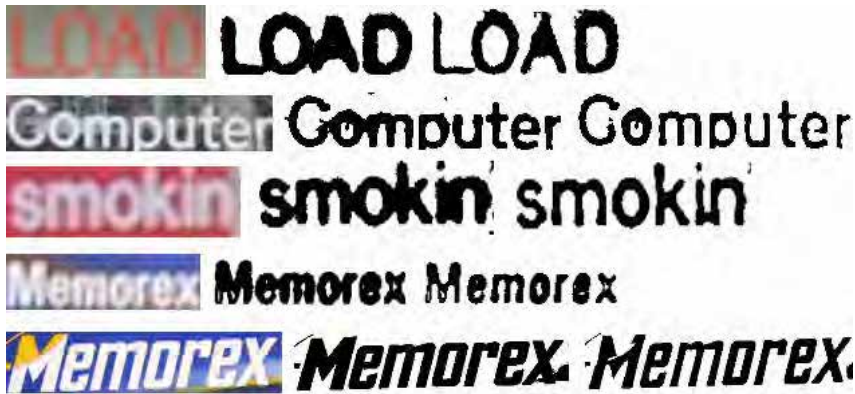
Fig. 10. Some character segmentation examples. From left to right: original image, SMC-based binary version and result after character segmentation.
