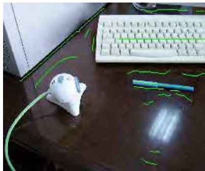
Fig. 4. Original image with the detected curvilinear skeletons (see Fig. 3). Several interesting objects as the ball pen, keyboard and webcam cable have been detected. Parameters used are: segmentation threshold = 95.0, U_{\Delta w} = 10 , \sigma_{\Delta w} = \sqrt{50} , U_w = 1.5 , U_{\Delta\alpha} = 30^\circ , L_{min} = 10 pixels.
