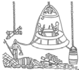
Fig. 1. Halley's diving bell, late 17th century. Weighted barrels of air replenished the bell's atmosphere. (U.S. Navy Diving Manual).
