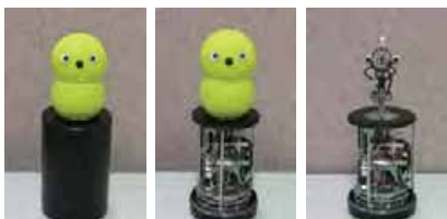
Fig. 4. Keepon’s simple appearance (left) and internal structure (middle/right).
