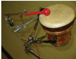
Fig. 15. Sample Motion Module Architecture: drumstick controlled by solenoid
