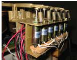
Fig. 11. Solenoid (with holding power of 1.5 pounds) attached to Jasche.
