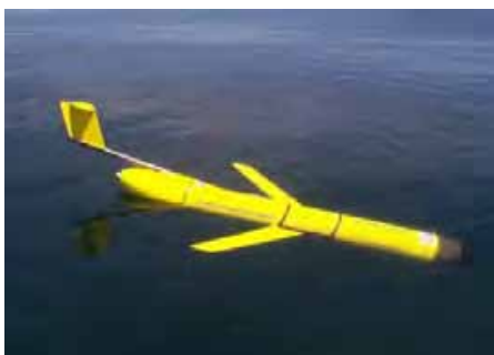
Fig. 12. The Slocum Glider, from Webb Research Corporation, Massachusetts, USA.
