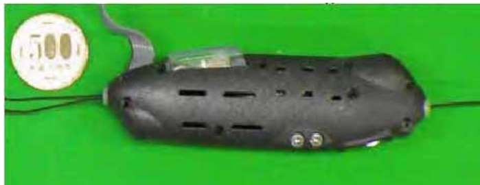
Fig. 2. A newly-developed, sensors-integrated muscle unit.
