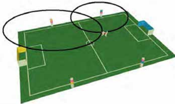
Fig. 6. Triangulation from two landmarks. By calculating distance to two different landmarks the robot can compute its position in the field.
