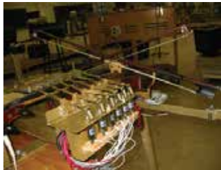
Fig. 14. Sample Motion Module Architecture: violin bow controlled by servo, violin string pressed by solenoids.
