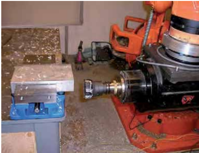
Figure 26. Robotic Milling Setup
