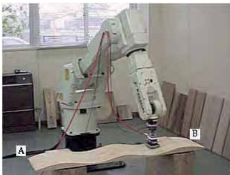
Photo 1. Robotic sanding system.
