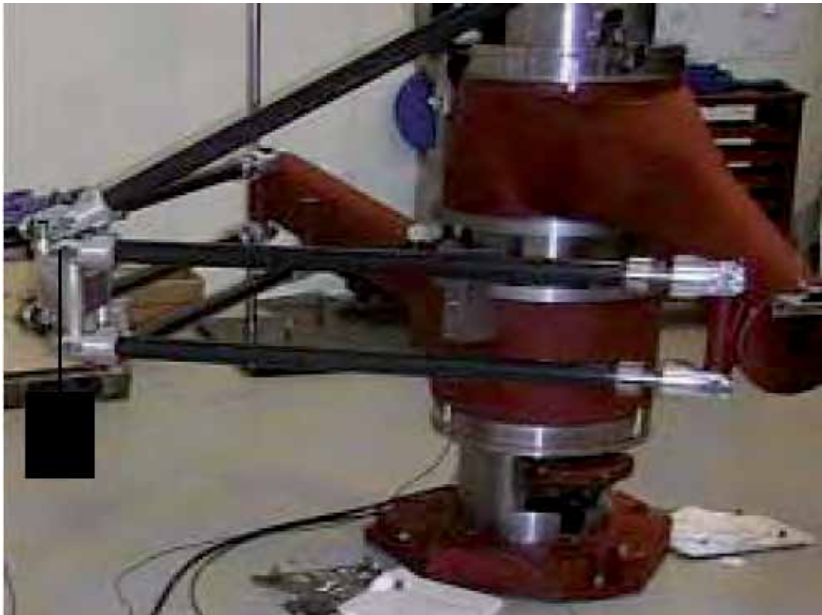
Figure 24. Setup of the TAU robot's Stiffness Measurement
