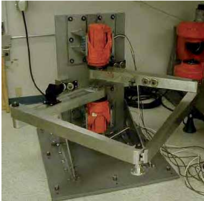
Figure 14. Two-Arm Test Platform (double SCARA structure)
