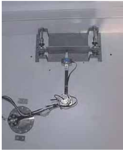
Figure 11. Top view of the 2-DOF robot and the nonrigid mechanical environment. (Reprinted from Baptista, L.; Sousa, J. & Sá da Costa, J. (2001b) with permission of Elsevier).
