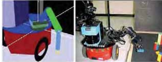
Fig. 20. a) Simulation of the robotic arm touching a point. b) Robot "Geometer" touching a point with its arm.
