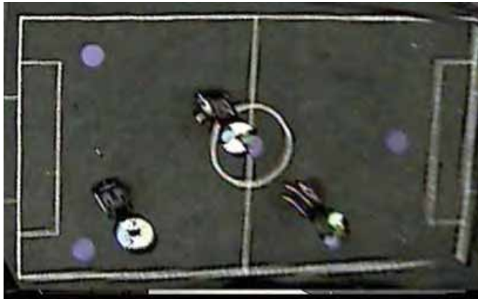
Fig. 4. Doraemon's overhead reconstruction (using average gradient interpolation) of the camera image shown in Fig. 1.
