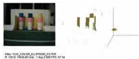
Fig. 3. Use of different bounding subspaces as color classes for classification of yellow in different color spaces. From left to right: Original image, Pixels from the original image classified as yellow, 3D representation of the color subspace. a) YUV Parallelepiped color class. b) RGB Cone color class. c) RGB Paraboloid color class. d) YUV Ellipsoid color class.
