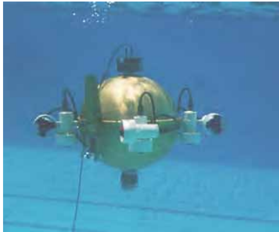
Fig. 11. Omni-Directional Intelligent Navigator (ODIN) vehicle.
