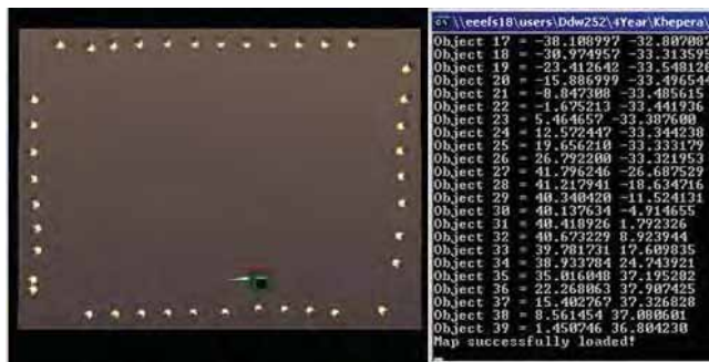
Fig. 8. Console output showing map objects being successfully loaded.
