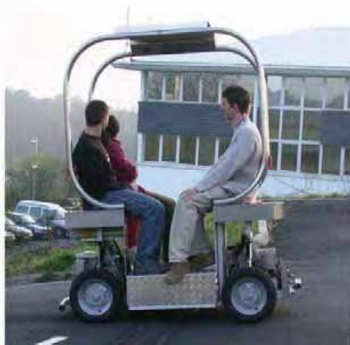
Fig. 9. Robucab mobile robot platform transporting four people.
