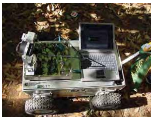
Fig. 2. Mobile robotic platform with computer-controlled scanner holding ultrasound transducer.
