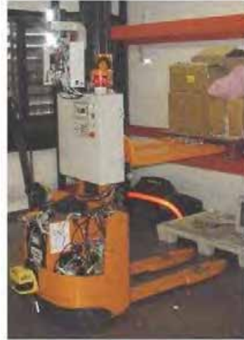
Fig. 5. Still EGV-10 robotized forklift used in a warehouse for real experimentation. Odometry, laser positioning and monocular vision data were recollected.
