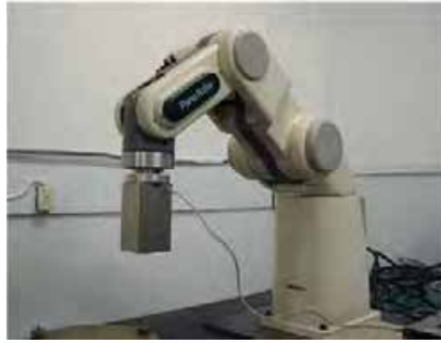
Fig. 4 .Robot equipped with the three-axis tactile sensor.
