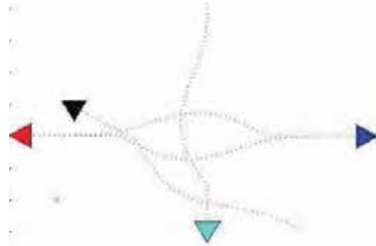
Fig. 15d. All Robots after avoiding collision go through their actual path.
