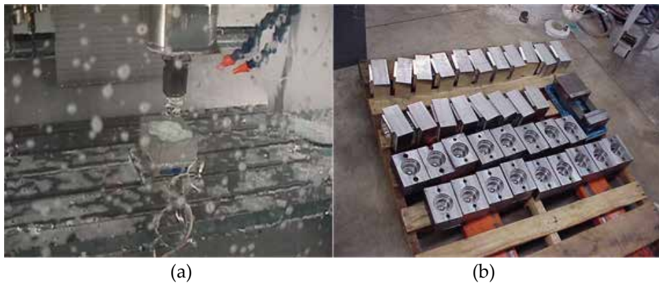
Figure 5. A snapshot of CNC machining (a) and a mixed array of parts consisted of 6061 Al (top), 7075 Al (middle), and 4140 medium carbon steel (the bottom two rows) (b).
