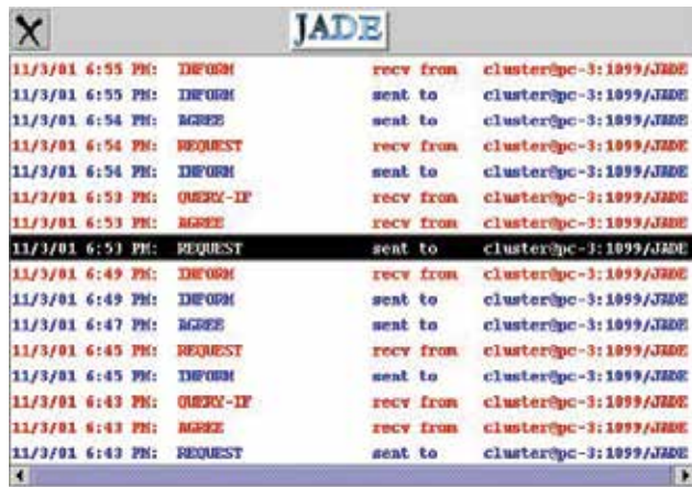
Figure 16. JADE Monitoring tool and messages between the Cluster and the Generic Agent
