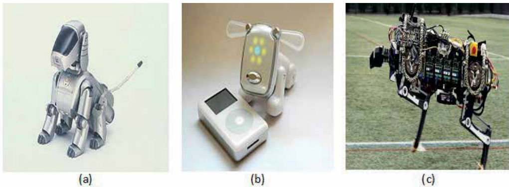
Figure 4. Zoomorphic robots: (a) AIBO, (b) iDog, (c) Cheetah.
