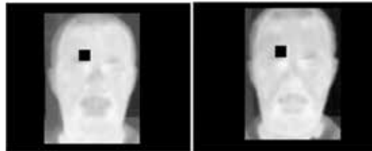
Figure 8. The same square region of 100 pixels on a pair of infrared images (sober-drunk) of a specific person.
