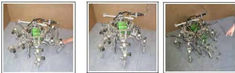
(a) Downward-motion of body (b) Upward-motion of body (c) Left-right motion of body
