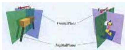
Fig. 7. Definition of sagittal plane and frontal plane.
