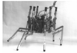
(f) Six-legged robot Silex (15 kg). Free University, Brussels.
