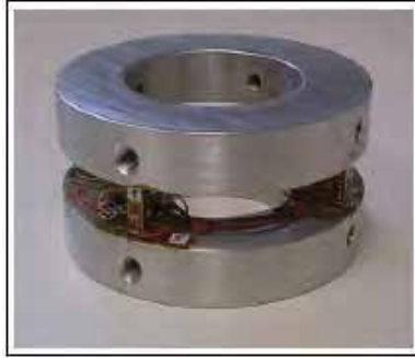
Fig. 3.6. Three-component force sensor for high loading.
