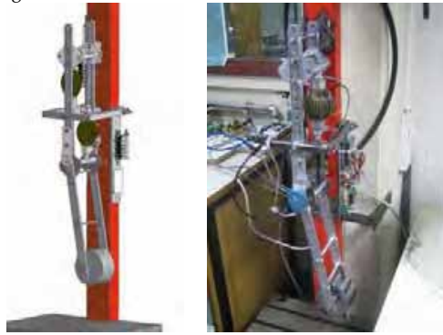
Fig. 7. CAD drawing and photograph of the pendulum setup.
