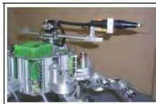
Fig. 3.5. Three-component force sensor mounted between the arm manipulator and a tool.
