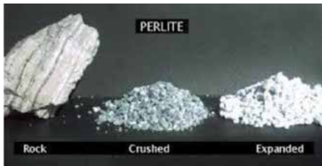
Figure 3. Morphology of perlite in its rock, crushed and expanded form.
