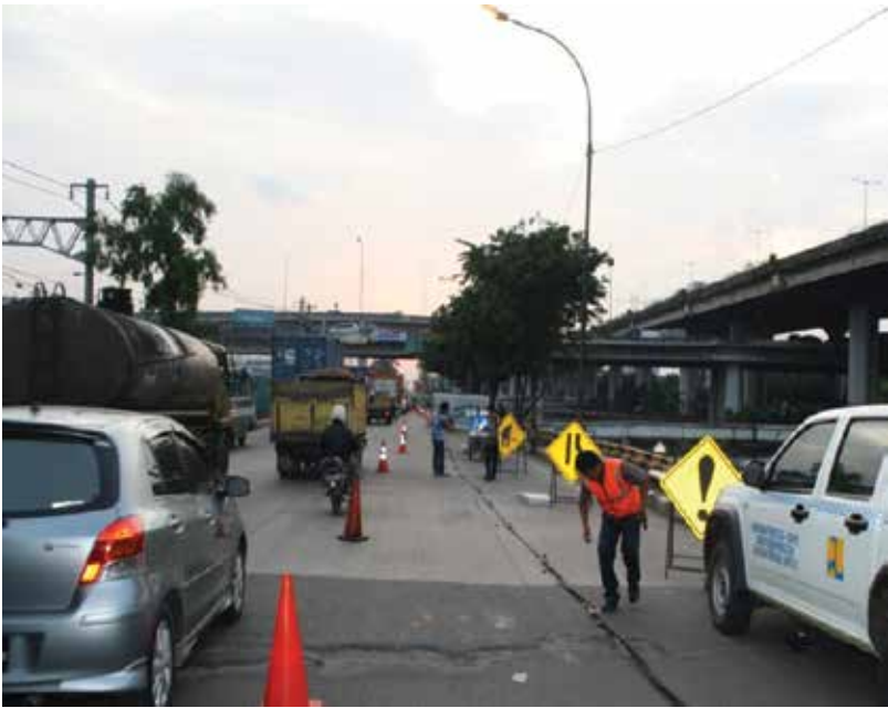
Figure 14. MASW data acquisition using land streamer on busy street.
