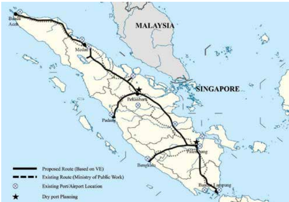
Figure 2. Conceptual design of Trans-Sumatera highway road. Source: [28].
