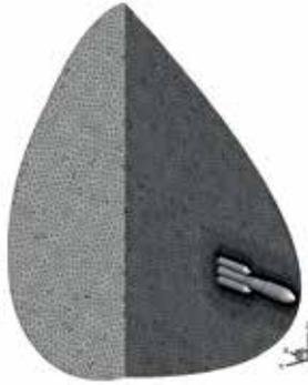
**Figure 11.** Overview of a hybrid mesh domain for sup-hypersonic CFD simulations.
