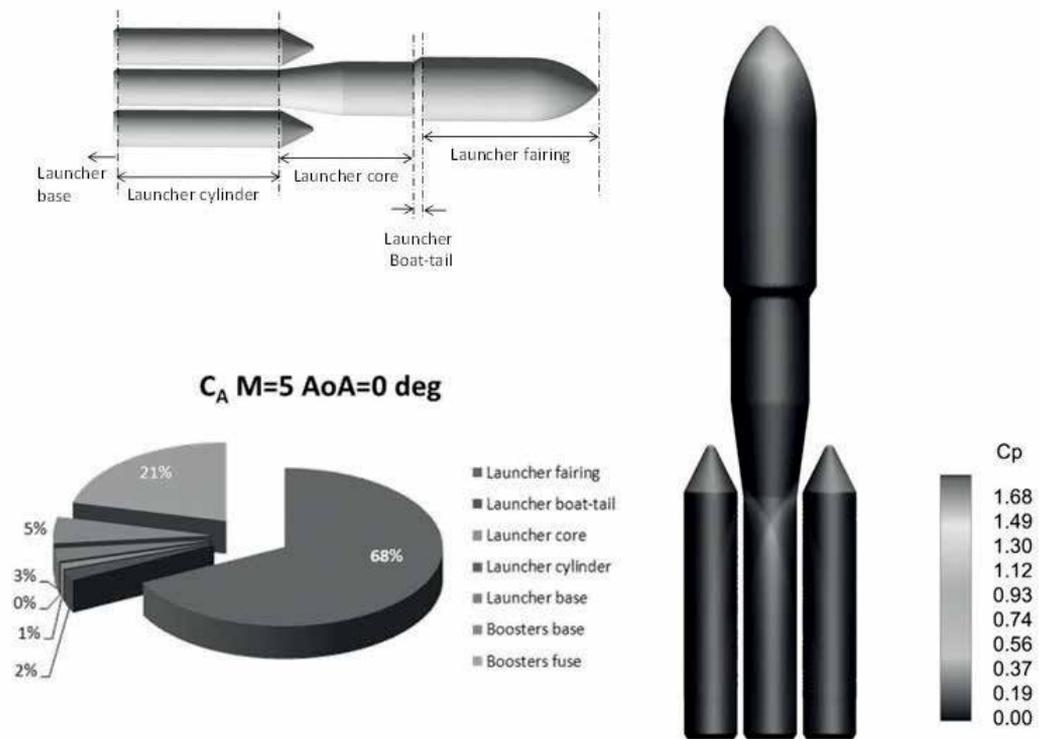
Figure 21.  $C_A$  breakdown at  $M_\infty = 5$  and  $\alpha = 0^\circ$ .
