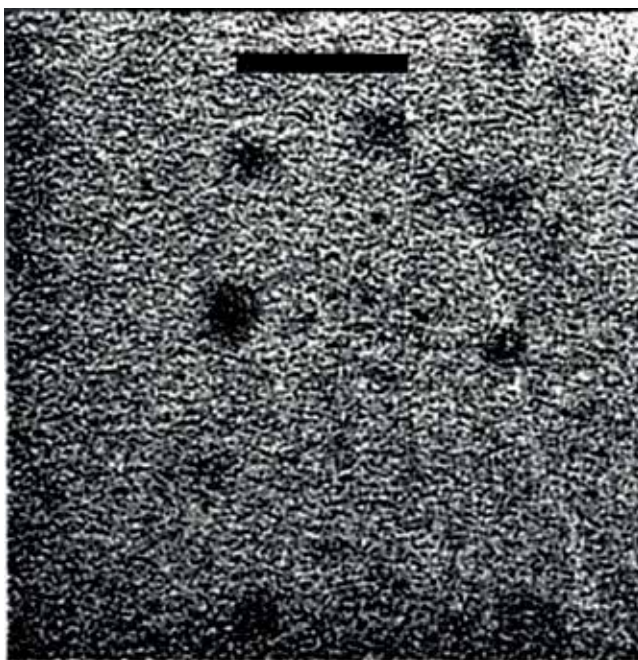
Figure 2. TEM image of GaN nanoparticles obtained from pyrolysis of \text{Ga}_2[\text{N}(\text{CH}_3)_2]_6 . Scale bar is 10 nm [43].
