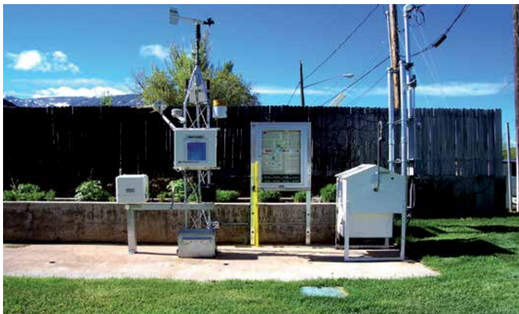
Fig. 4. A typical CEMP environmental monitoring station, with a full suite of meteorological sensors, radiation detection equipment, air sampler, and interpretive display with real-time sensor readouts.
