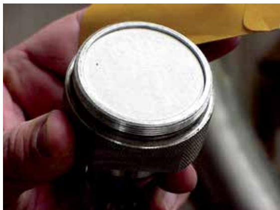
Fig. 2. Fixed head radioactive air stack sampler with 47-mm diameter filter in place
