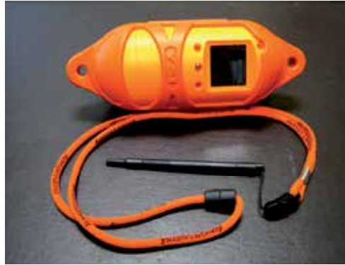
Fig. 9. The YSI CastAway CTD profiler and magnetic stylus.
