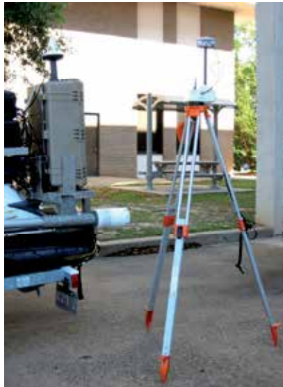
Fig. 2. SonTek/YSI RiverSurveyor M9 ADCP and RTK DGPS base station.
