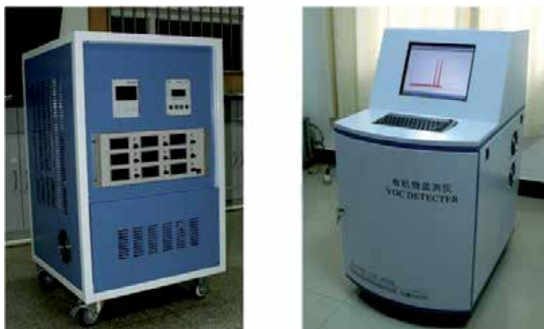
Fig. 9. A series of PTR-MS instruments developed for different requirements.
