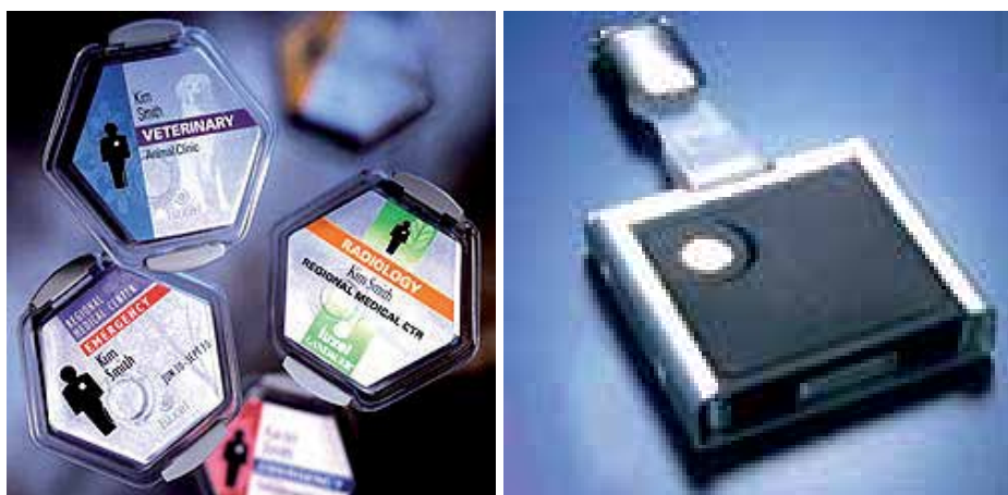
Fig. 7. Photographs of the OSL dosimeter (Type S) as shown the left photo picture and of the DIS dosimeter (Type DIS-1) as shown in the right photo picture.
