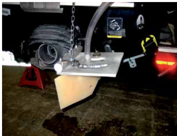
Fig. 8. The custom-designed center-point swivel and ram intake for the YSI PSK.
