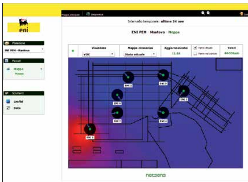
Fig. 20. Bi-dimensional map representing VOC concentration in the plant
