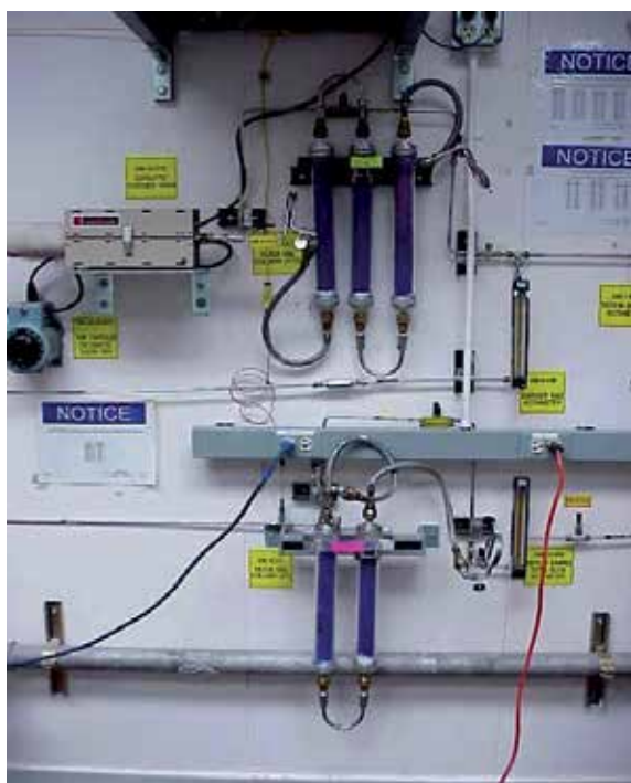
Fig. 3. Silica gel columns in use for tritium sampling system; three columns are used for collecting water vapors, and then the dry gas goes through a catalyst to form the water vapor collected using the two columns (Barnett et al., 2004)
