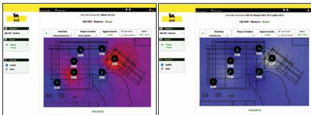
Fig. 19. Bi-dimensional map of air temperature (left) and air RH (right) distribution in the area of the plant
