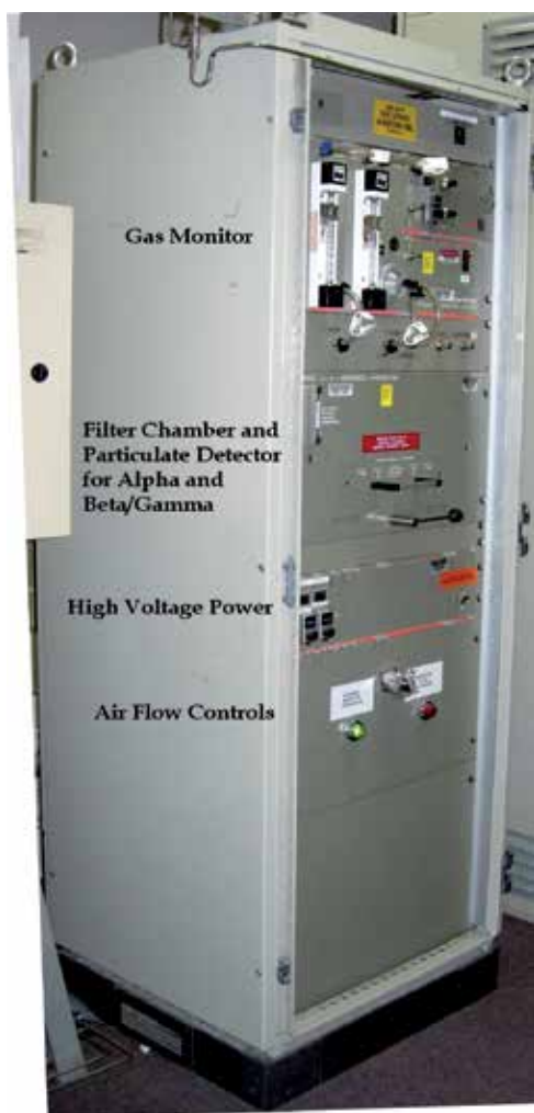
Fig. 4. Combination continuous air monitor for particulates and gases
