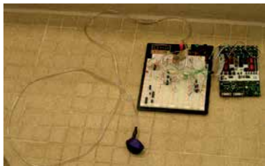
Fig. 16. Pressure sensor. Note balloon and tubing.
