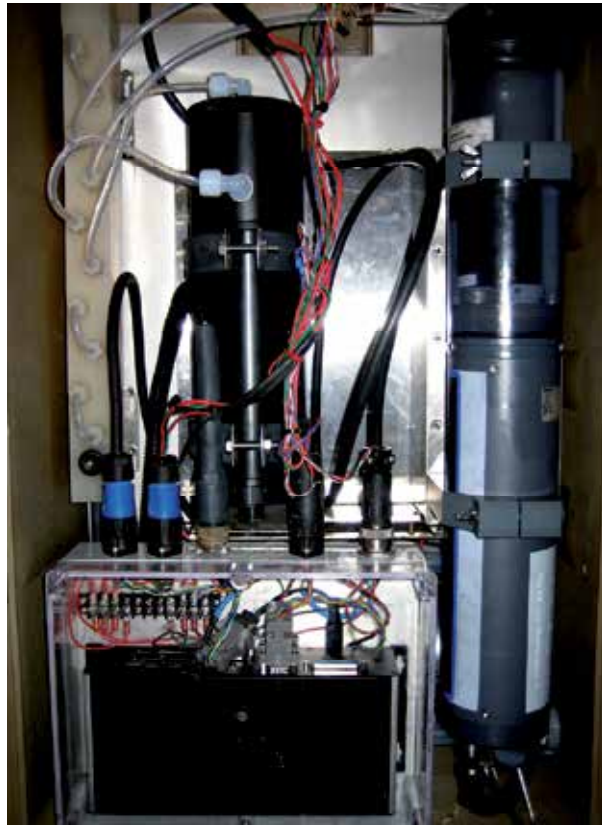
Fig. 7. Internal components of the YSI PSK system. The YSI sonde is on the right, the Turner Designs fluorometer is the black cylinder, the flow manifold is on the left, and the onboard PC is at the bottom. The diaphragm pump is hidden behind the PC.
