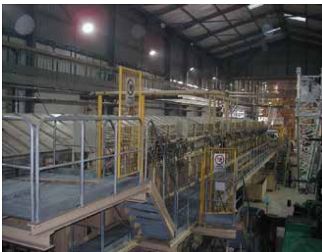
Fig. 6. Continuous press in a particleboard plant (courtesy from Sonae Indústria, Portugal).
