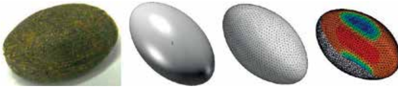
Figure 7. Jatropha curcas L. seed (CAD model, FEM model, and simulation model).
