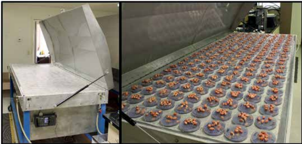
Figure 3. Thermal gradient table (left) and peanut seed after evaluation for germination (right).
