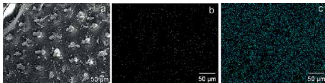
Figure 5. Prosthernum of S. oryzae : a – SEM image of S. oryzae exposed to untreated wheat kernels (400×); b – exposed to wheat kernels treated with 125 ppm DE, silicon (Si) counts from Energy Dispersive Spectroscopy (EDS); c – exposed to wheat kernels treated with 125 ppm NSA, aluminum (Al) counts from EDS. Format JEOL/EO, Version 1.0; Instrument JSM-6610; Acc. Volt 10; Mag 400; Spot Size 35; Vac Mode HV. c – Aluminum (Al) counts from Energy Dispersive Spectroscopy (EDS) – Filter Fit \chi^2 value: 31.161; Errors: \pm 2 ; Sigma Correction Method: Proza (Phi-Rho-Z); Acc. Voltage: 12.0 kV; Take off angle: 35.9°.
