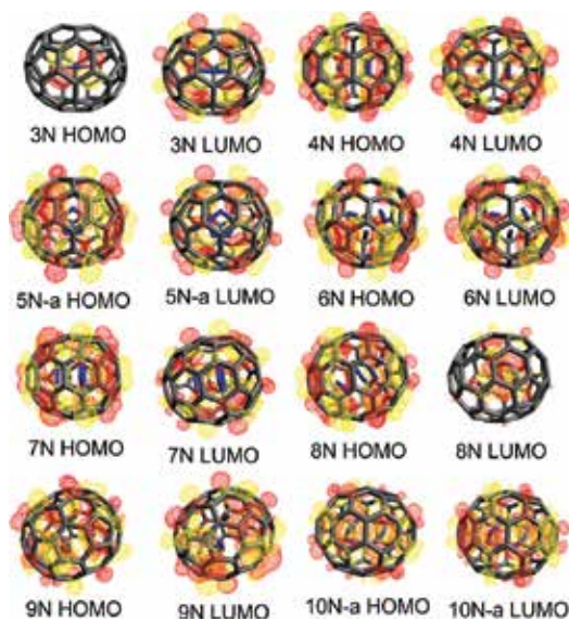
Figure 4. Frontier orbitals for N_n@C_{70} where n = 3-10 , endohedral fullerenes, calculated using the B3LYP/6-311G method.
