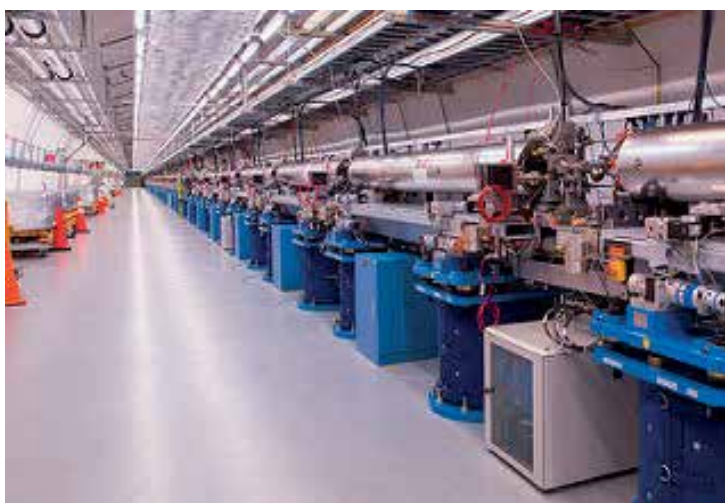
Figure 1. Schematic of the 33 m long LCLS FEL undulator [34].
