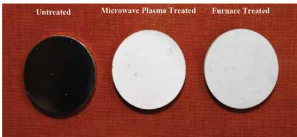
Figure 9. Photograph of oxide-layer formed on the 25-mm diameter titanium disc using microwave plasma and air furnace. Reprinted from [64] with permission from Elsevier.
