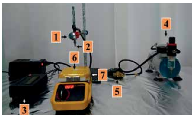
Figure 1. Image of the experimental setup for ZnO, CZTS, and CZT films deposition by pulsed spray pyrolysis: (1) spraying gun with initial precursor volume reservoir, (2) spraying nozzle, (3) microcontroller block, (4) compressor, (5) electromagnetic valve, (6) substrate, and (7) heating plate [18, 19].
