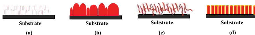
Figure 12. Morphologies of manganese oxide film formed at annealing temperature of (a) 100 – 200°C, (b) 300°C, (c) 500°C, and (d) 600°C.
