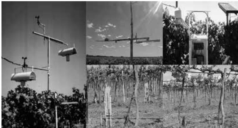
Figure 2. Measurements of gradients of air temperature, vapor pressure and wind speed; incident and reflected shortwave; net radiation; acquisition data system; and soil moisture in Bowen ratio system of wine grape.
