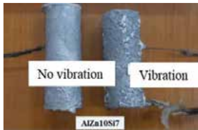
Figure 16. Photographs showing the roughness of the samples in AlZn10Si7 alloy with and with no vibration [10].
