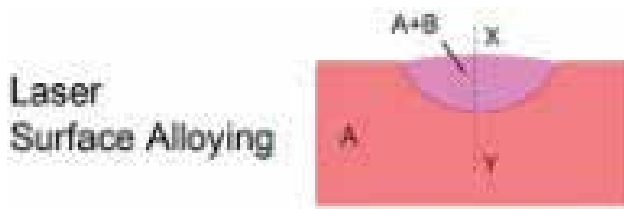
Figure 3. Schematic diagram displaying laser surface alloying [15].
