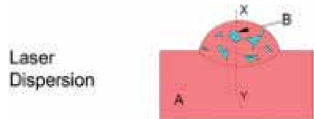
Figure 5. Schematic diagram showing the surface metal matrix formed by laser dispersion [15].
