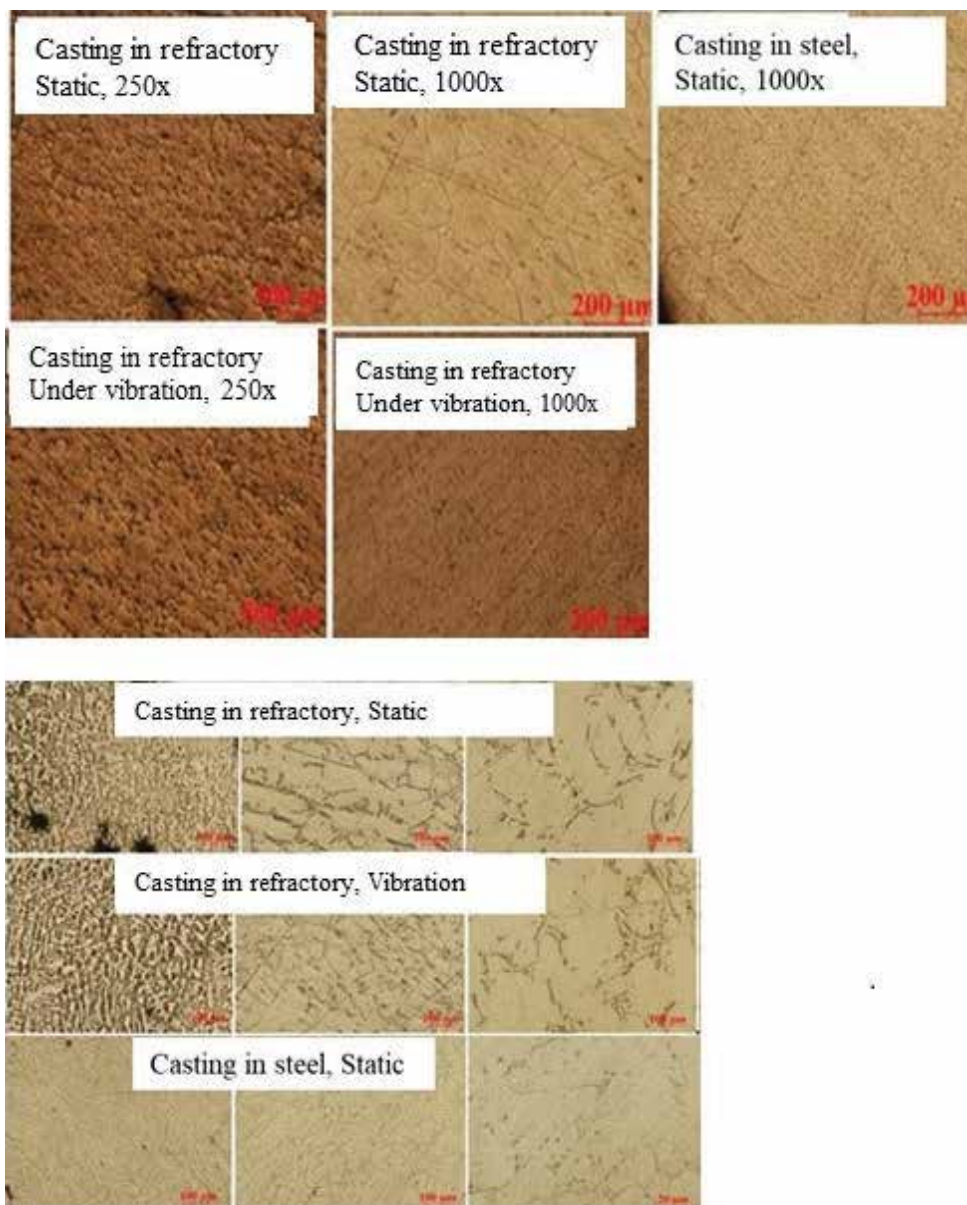
Figure 11. OM microstructure of the AlCu4 alloy (top) and AlSi7Mg0.3 (bottom) casted in different dies and with no vibration and under vibration [10].
