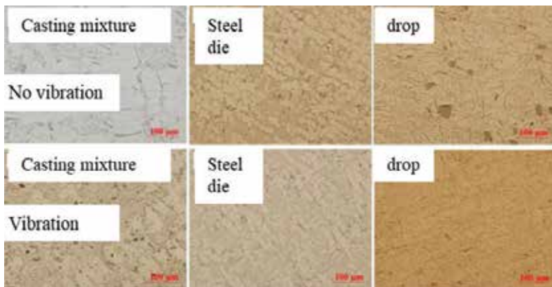
Figure 23. OM microstructure of the AlSi12CuMgNi alloy in different casting conditions [10].
