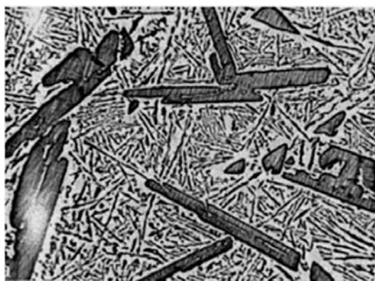
Figure 1. Primary Si in the form of a plate in Al-20%Si [8].
