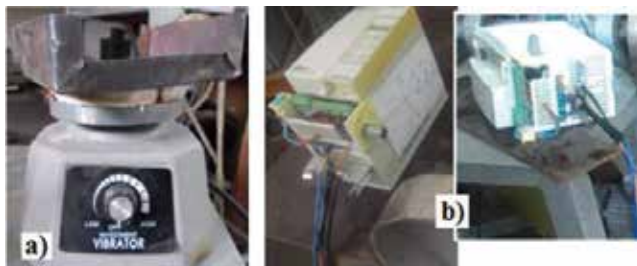
Figure 4. The set-up used experimentally for the mechanical vibration of the melt (a) and command block used for the variation and the registration of the frequency (b) [10].
