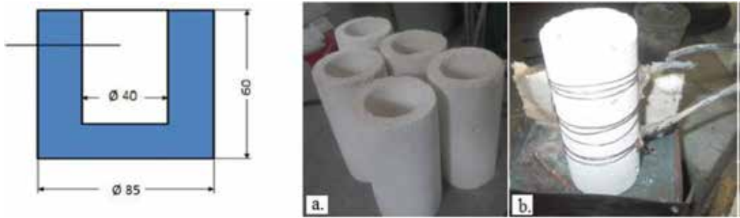
Figure 5. The shape and the size of the forms used for the casting; (a) crucible in refractory material and (b) thermocouples placed for monitoring the cooling [10].
