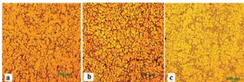
Figure 22. OM microstructure of the AlSi 7 Mg 0.3 alloy: (a) with no rotator electromagnetic field and under rotator electromagnetic field, (b) top surface and (c) middle part of the sample [8, 10].
