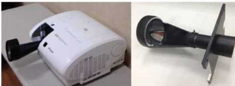
Figure 19. Utmost Co. LCoS projection engine with the self-designed optics and opto-mechatronic mount.
