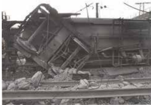
Figure 8. Plowing mechanism of the track by the bogie of the overturned carriage.
