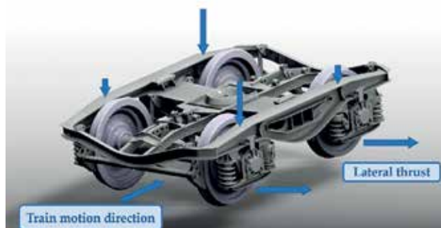
Figure 2. Forces acting on the first bogie of carriage no. 1 after breakage of the second axle (rear wheelset) due to fatigue failure externally with respect to the left wheel.
