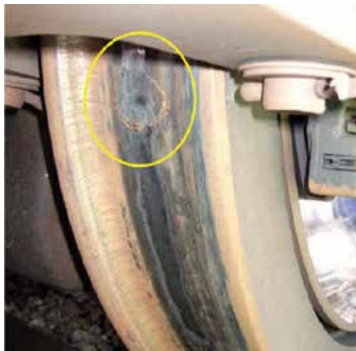
Figure 1. Photograph of a wheel flat formed by wheel-rail sliding [6].
