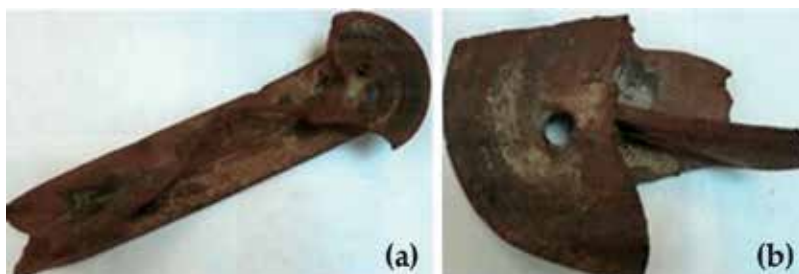
Figure 26. Two of the three chunks of the right axle box of the front wheel set of the front bogie of carriage no. 1: (a) chunk of the axle box found between the rails near the deformed check rail and (b) chunk of the axle box greatly abraded by the granite sidewalk curb exerting a grinding action on the right axle box, found externally to the track near the right-side rail in the train motion direction.
