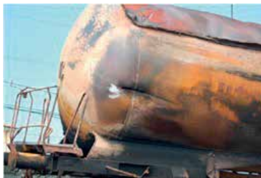
Figure 9. Carriage no. 1 with a cut opening on the tank shell.
