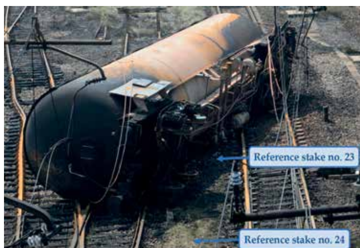
Figure 13. Rear view of carriage no. 1 in the accident scene and positions of track reference stake nos. 23 and 24.
