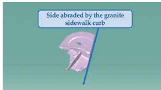
Figure 27. Digital twin of the chunk of the right axle box of the first wheel set of the front bogey of carriage no. 1 obtained by reverse engineering reconstruction based on geometry acquisition with a structured light optical sensor.
