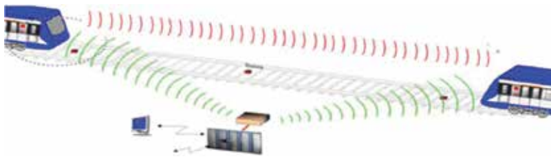
Figure 12. Schematic of the V2V-CBTC with both a direct link between trains and a train-to-infrastructure link.
