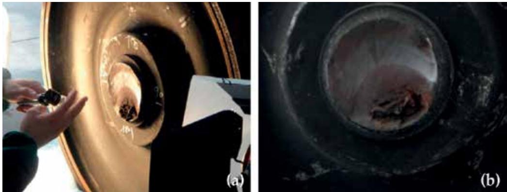
Figure 1. (a) Fatigue failure of the fracture surface of the axle on the wheel side. (b) Presence of a smooth area related to the slow propagation of the fatigue crack and of a rougher area of rapid failure of the residual axle section.
