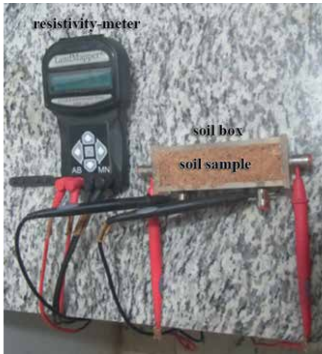
Figure 3. LandMapper of Landviser and Miller soil box used for the measurement of the electrical resistivity of each soil sample in laboratory, according to ASTM standard G57-06 (photo courtesy of 3P Soc. Ltda).
