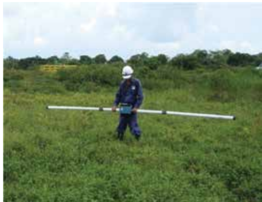
Figure 2. EM31-MK2 ground conductivity meter in field operations [12].
