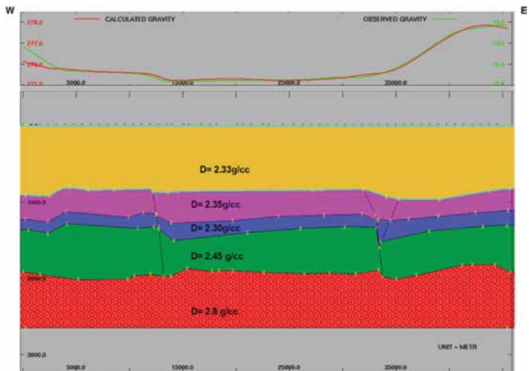
Figure 6. 2D gravity model across the Tangent fault as well as a smaller fault to the east. Layer boundaries are defined based on seismic profile data ( Figure 5 ). These faults appear to have a subtle gravity response.
