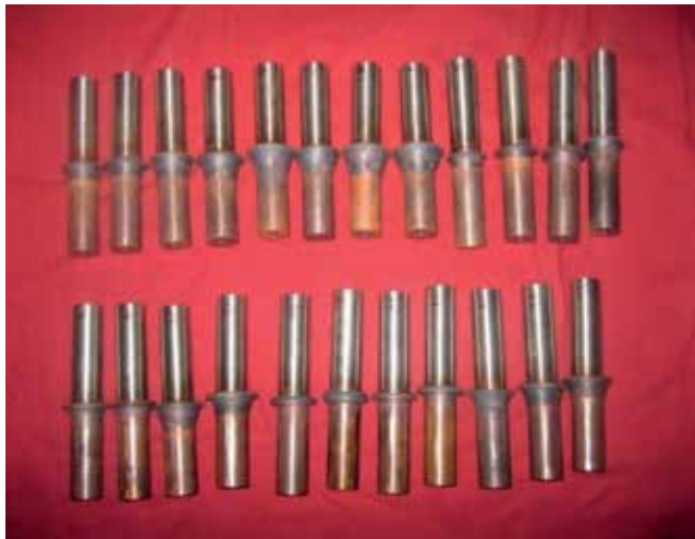
Figure 1. 304L SS-Cu welded joints.
