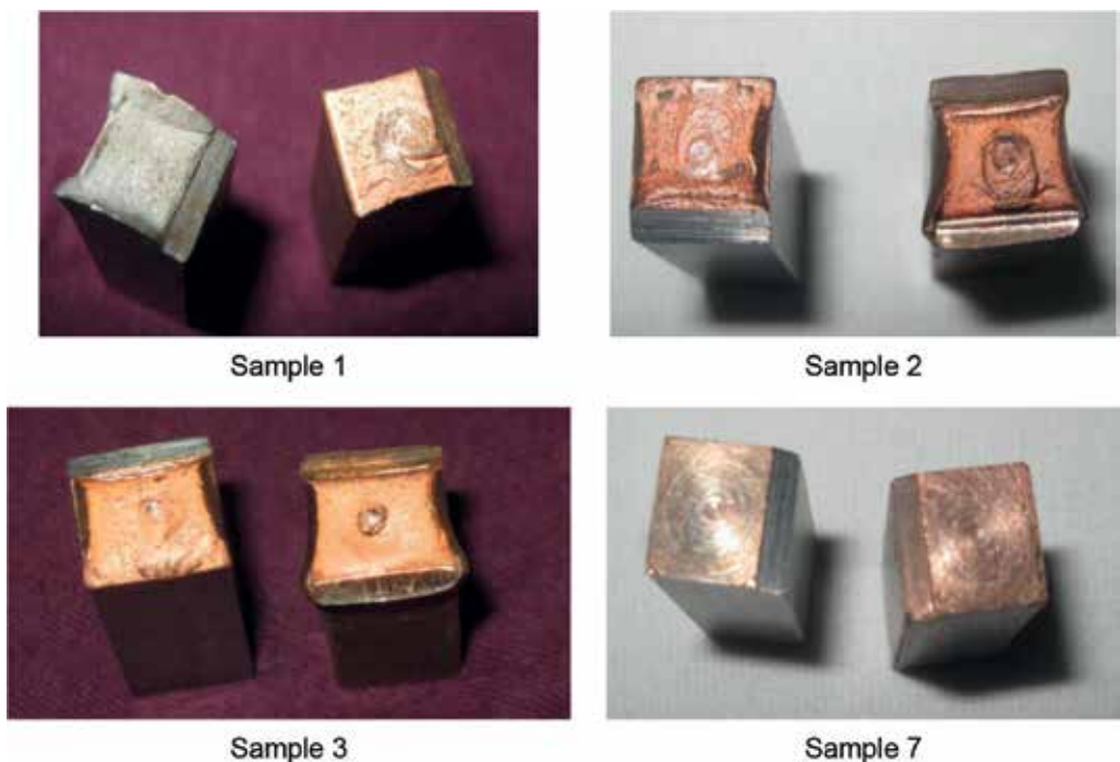
Figure 5. Impact tested samples on 304L-Cu joint.
