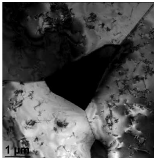
Figure 12. The \sigma phase precipitation at the contact point of three grain boundaries in T321H steel after long-term service.
