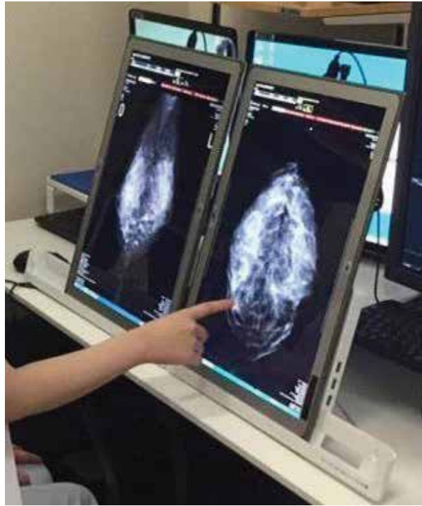
Figure 2. Two sets of 4K tablet PCs with high-resolution color monitors (4K UT-MA6, 2560 × 3840 pixels, 20.8 inch; Panasonic).
