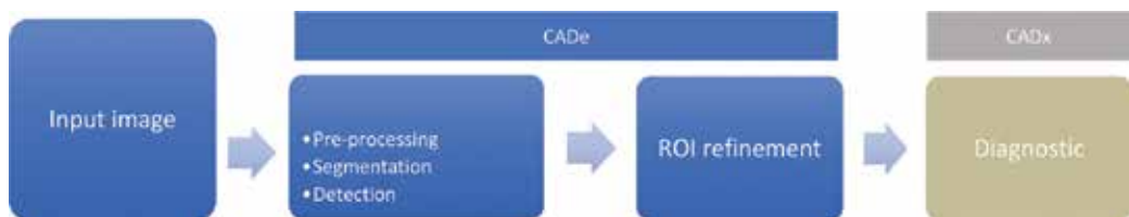
Figure 1. Typical workflow of a CADe/CADx system, adapted from Chen g et al. [13].
