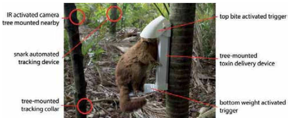
Figure 4. Field trial devices configured to capture firing event data, including date, time, and location and snapshot evidence.
