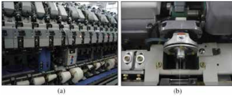
Figure 2. MVS 861 spinning machine: (a) the general view of the machine, (b) the yarn spinning unit.
