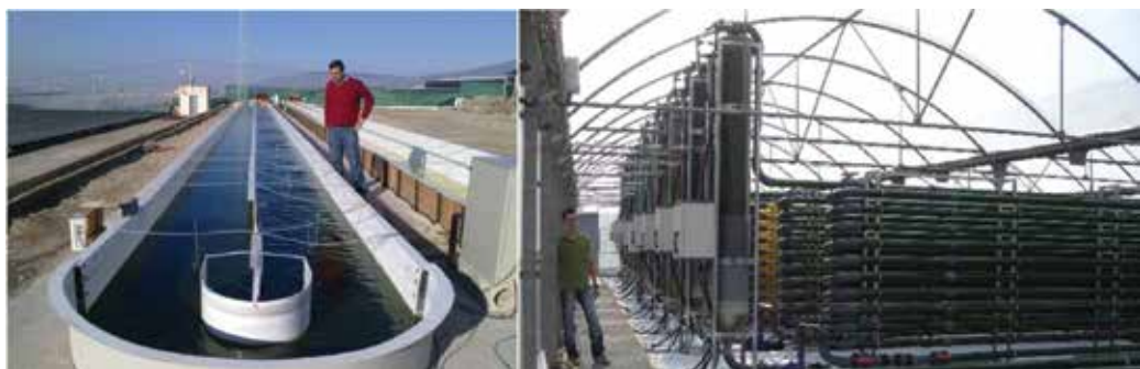
Figure 4. Image of some photobioreactors used for outdoor production of microalgae at a large scale. A raceway reactor of 20 m 3 as an example of open reactor (left side) and ten tubular reactors of 30 m 3 as an example of tubular reactors (right side). All of them installed and operated at Estación Experimental Las Palmerillas (Fundación Cajamar), Almeria, Spain.
