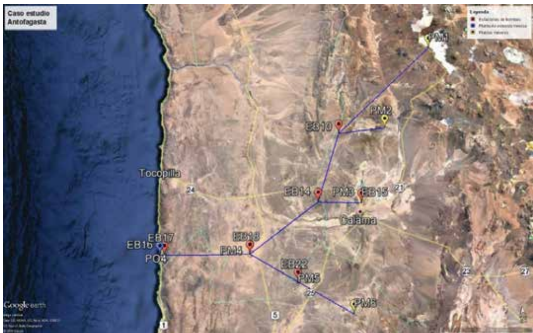
Figure 11. Optimum proposed model of an integrated desalinated water supply system for six mining plants in the Antofagasta region. PO indicator: reverse osmosis plants; EB indicator: pumping stations; and PM indicator: mining plants [14].
