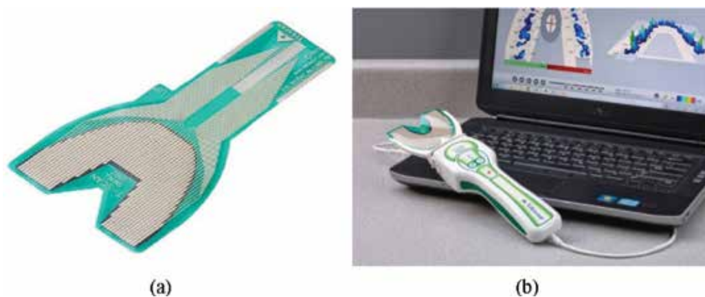
Figure 8. (a) The T-Scan Novus Definition (HD) sensor records 256 levels of relative occlusal force in 0.003 s time frames to reveal an occlusal playback video that illustrates changing occlusal force levels across time. (b) The T-Scan Novus recording handle with the HD sensor in place, connected directly to a computer with a USB plug.
