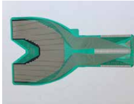
Figure 23. The T-scan sensor is an ultra-thin (0.004 inch, 0.1 mm), flexible printed circuit that detects your patient's occlusal forces. These sensors are made up of 1370 active pressure sensing locations for the large sensor (#2002 for the Novus Handpiece, and #2001 for the Evolution Handle), and 1122 pressure sensing locations for the small sensor (#2502 for the Novus Handpiece, and #2501 for the Evolution Handle). These sensing locations are referred to as "sensing elements" or "sensors." the "sensors" are arranged in rows and columns on the sensor. Each sensel can be seen as an individual square on the computer screen by selecting the 2D display mode (text is from company user manual, Teksan Inc. USA) [95] ( Figures 24 and 25 ).
