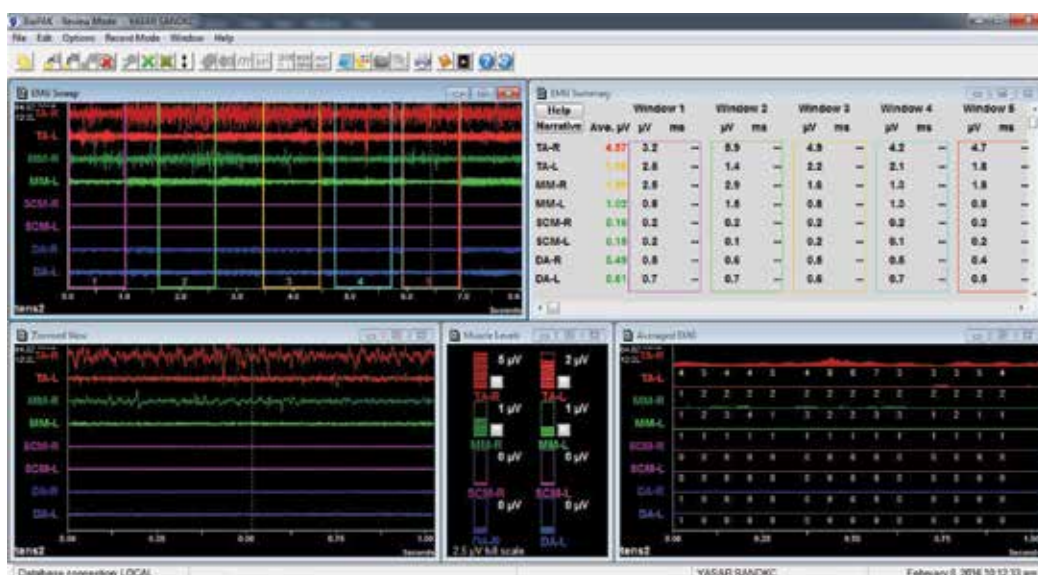
Figure 6. Both the temporalis and masseter muscle electrical activity levels are higher than the physiological average resting values. This is not unexpected during the development of new prosthesis adaptation.
