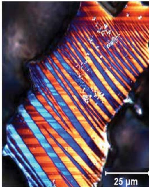
**Figure 15.** Optical micrograph of twins in Ni-Mn-Ga foam, extending entirely from pore to pore (black) [10].
