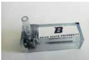
**Figure 28.** Micro-pump created based on Ni-Mn-Ga alloys [111].
