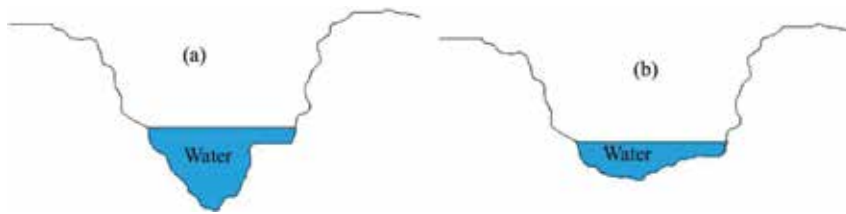
Figure 3. Two river cross sections. Cross section (a) is derived from LIDAR-based DEM while (b) is derived from ASTER GDEM.
