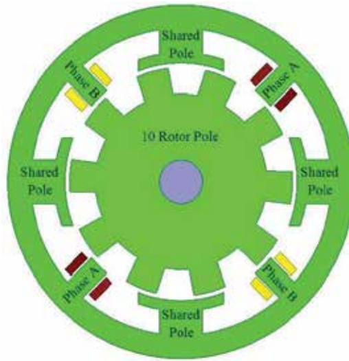
Figure 16. A common pole E-core SRM configuration.
