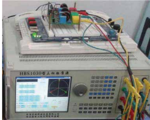
Figure 2. Measurement scheme for the laboratory experiment of the proposed method.
