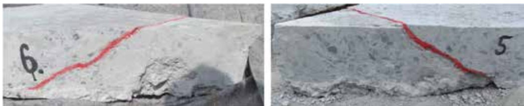
Figure 8. Diagonal cuts of slab.
