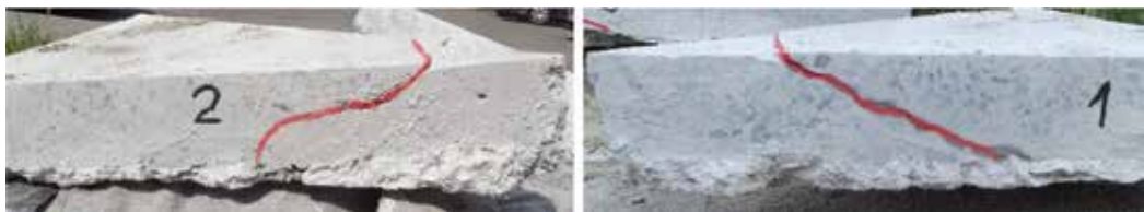
Figure 7. Lateral cuts of slab.
