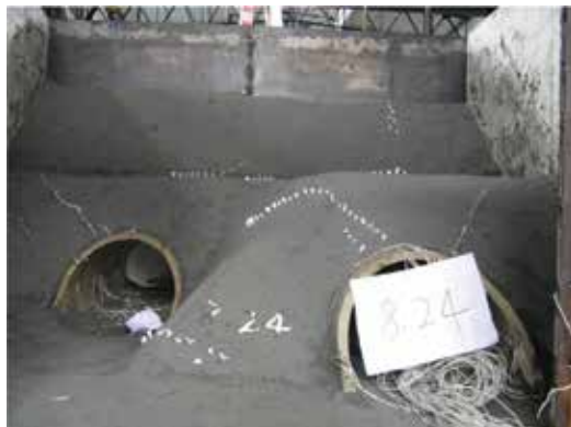
Figure 12. The distribution of ground cracks with soft isolation layer.
