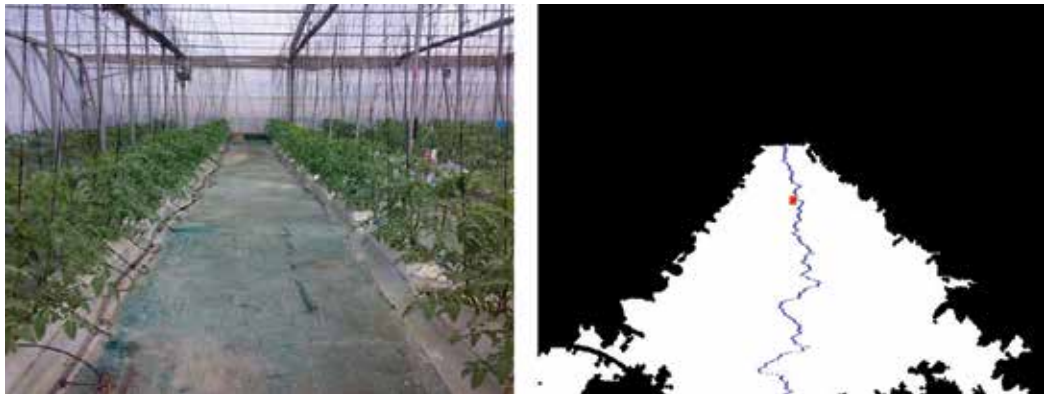
Figure 4. An example of a segmented corridor marking the trajectory to follow by the Fitorobot.
