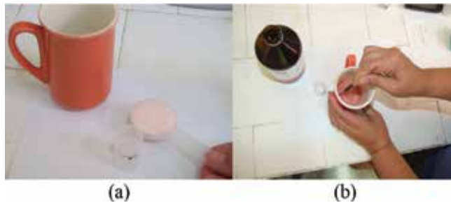
Figure 1. (a) Heat-curing acrylic powder and liquid and (b) mixing the acrylic paste.
