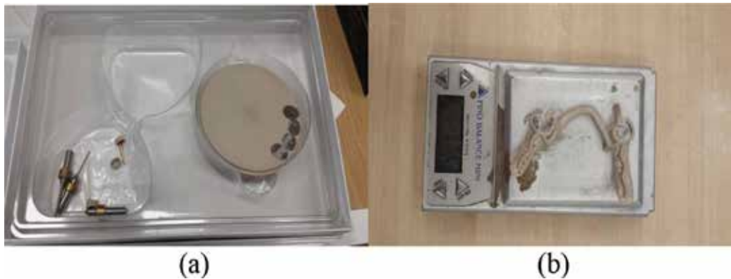
Figure 21. (a) PEEK milling disk and (b) PEEK framework on a weighting scale.
