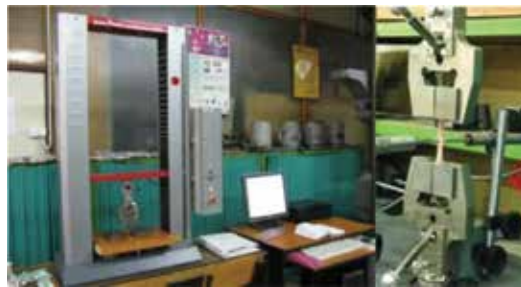
Figure 5. The determination of tensile mechanical resistance using the Zwick Roel extensometer.
