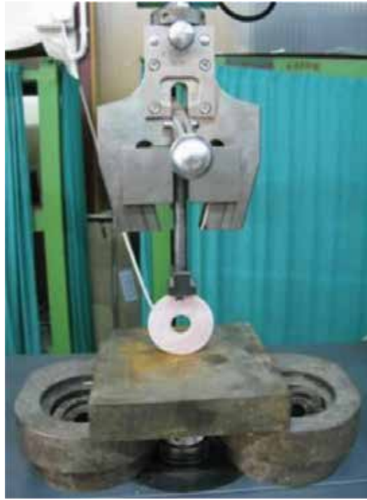
Figure 10. Meliodent sample during compression experiment.
