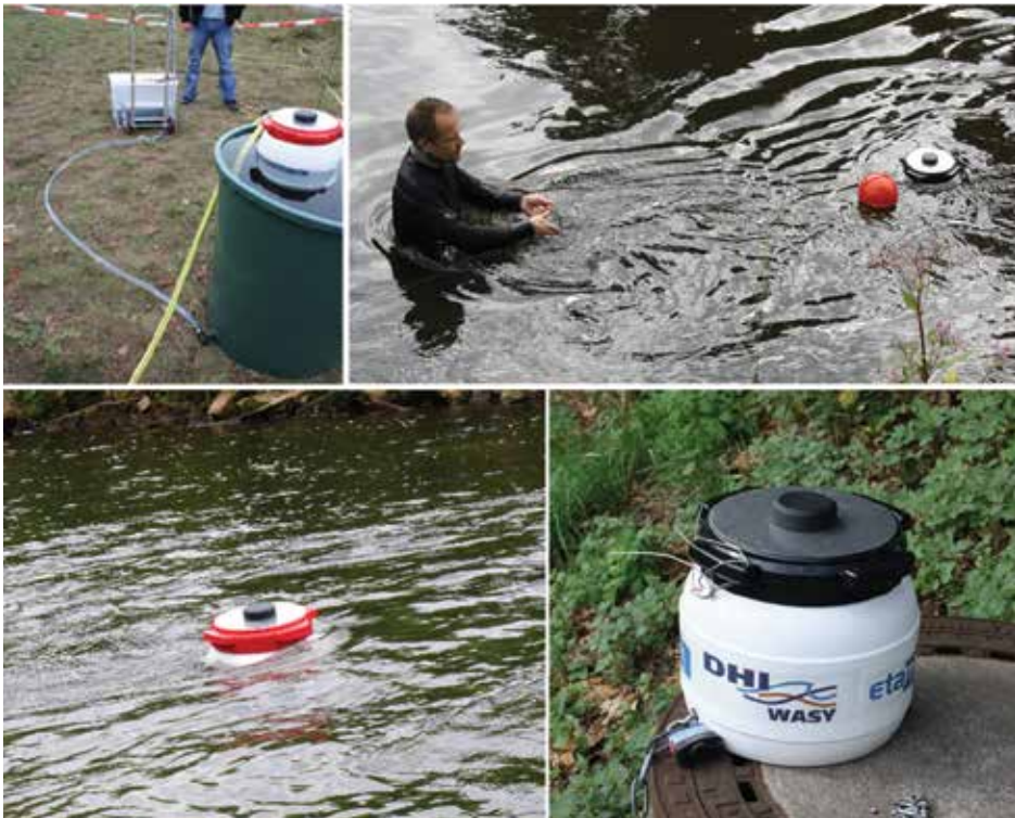
Fig. 2. Deployment of a G-WaLe floater in a river.
