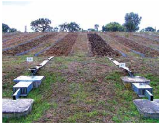
Figure 2. Plots to evaluate soil erosion by water under some crop rotations (Experimental Station in Polytechnic Institute of Castelo Branco/School of Agriculture).
