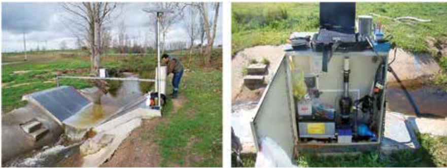
Figure 8. Hydrometric and water quality station located at the outlet of the study catchment.
