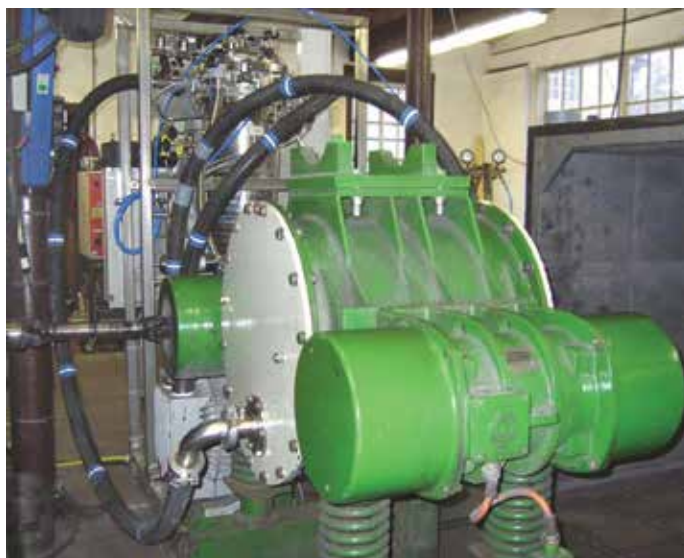
Figure 1. Industrial eccentric vibratory mill (type: ESM 656–0.5 ks, Siebtechnik GmbH, Germany).
